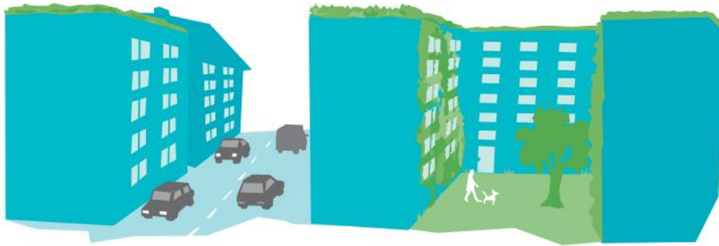
Green roofs with short vegetated roof-edge barriers
